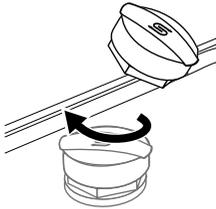
Turn the cap of the salt container clockwise to close the salt container.
