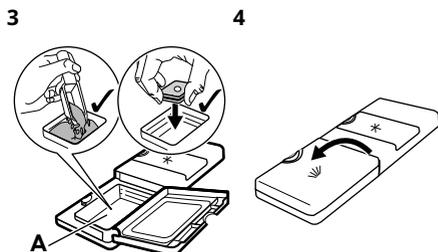
Put the detergent or the multi-tablet in compartment (A).
