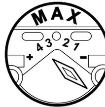
To adjust the released quantity of rinse aid, turn the selector between position 1 (lowest quantity) and position 4 (highest quantity).
