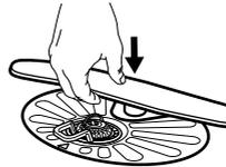
To install the spray arm back, press it downwards.
