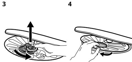
To remove filters (B) and (C), turn the handle counterclockwise and pull it upwards. Remove the filter (C) out of filter (B). Wash the filters with water.
