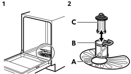
Make sure that there are no residues of food or soil in or around the edge of the sump. The filter system is made of three parts.
