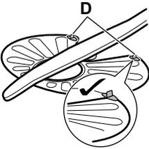
Put the flat filter (A) back in place. Make sure that it is correctly positioned under the 2 guides (D).
