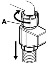
Disconnect the hose. Turn the fastener A clockwise.
