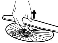
To remove the lower spray arm, pull it upwards.
