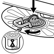
Reassemble the filters (B) and (C). Put them back in the filter (A). Turn the handle clockwise until it locks.
