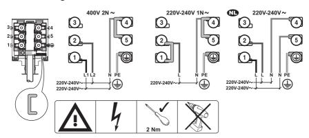
insert the shunts between the screws as shown.
