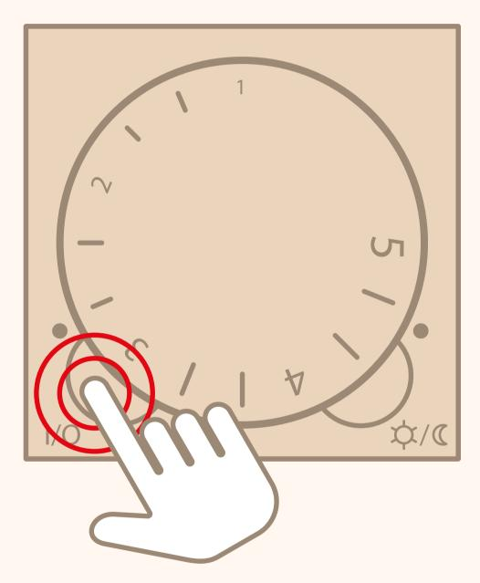
By pressing the I/O button, you can activate the floor heating.
